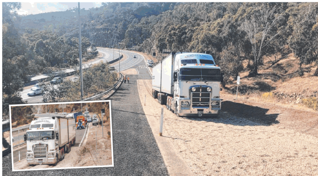
SCARY: After its brakes failed yesterday, this truck was forced to use an arrester bed at Mt Osmond to avert disaster on the freeway. Picture: BEN HARVY
